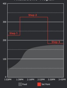
The graph above shows a 3 Step Program. Step 1 is hold setpoint of 225°F for 20 minutes. Step 2 is to hold a setpoint at 325° until target temp reaches 165°. Step 3 is hold setpoint at 180°, which is the default hold step that is added at the end of programs.
